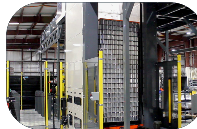
Empty cans infeeding into the system
