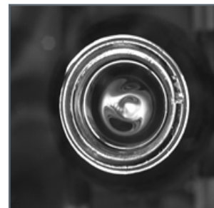
Chipped sealing surface
